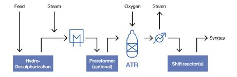
ATR based smart syngas solution: Lurgi Megasyn  $^{\text{TM}}\text{-}$  applied since 2002
