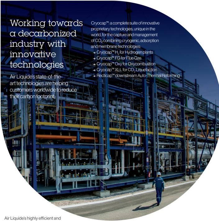
Air Liquide's highly efficient and robust technology, Cryocap™, operating at large scale for more than 5 years in Port Jerome, France, enables the capture of CO₂ from a hydrogen production unit via a combination of cryogenic and membrane processes.
