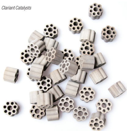
FIGURE 5. The eight-hole flower-like shape of the ReforMax LDP series catalyst is designed to optimize catalyst geometry and mechanical strength, and results in a reduced pressure drop across the reactor tubes
